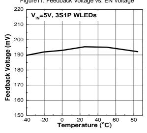
Figure13. Feedback Voltage vs. Temperature.
