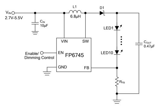
Figure 2. Typical Application Circuit of FP6745
