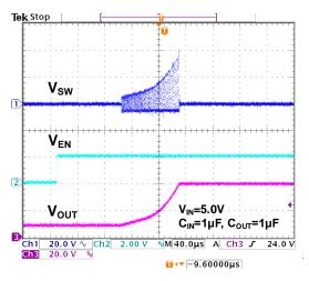
Figure 9. Open load Protection Waveforms
