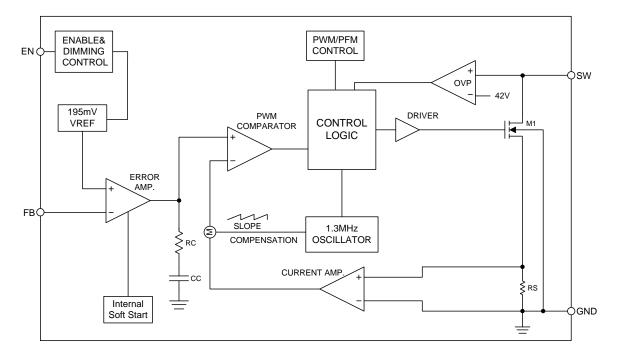
Figure 3. Block Diagram of FP6745
