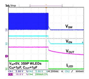
Figure 6. Enable Shutdown Response Waveforms
