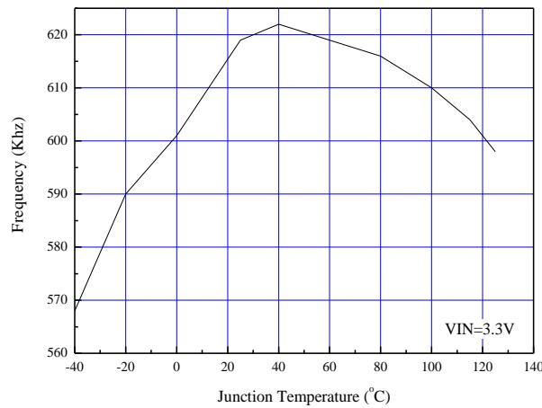
Figure 6. Frequency vs. Junction Temperature
