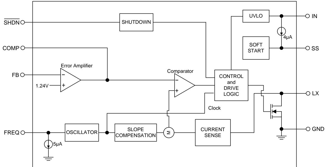
Figure 3. Block Diagram of FP6795
