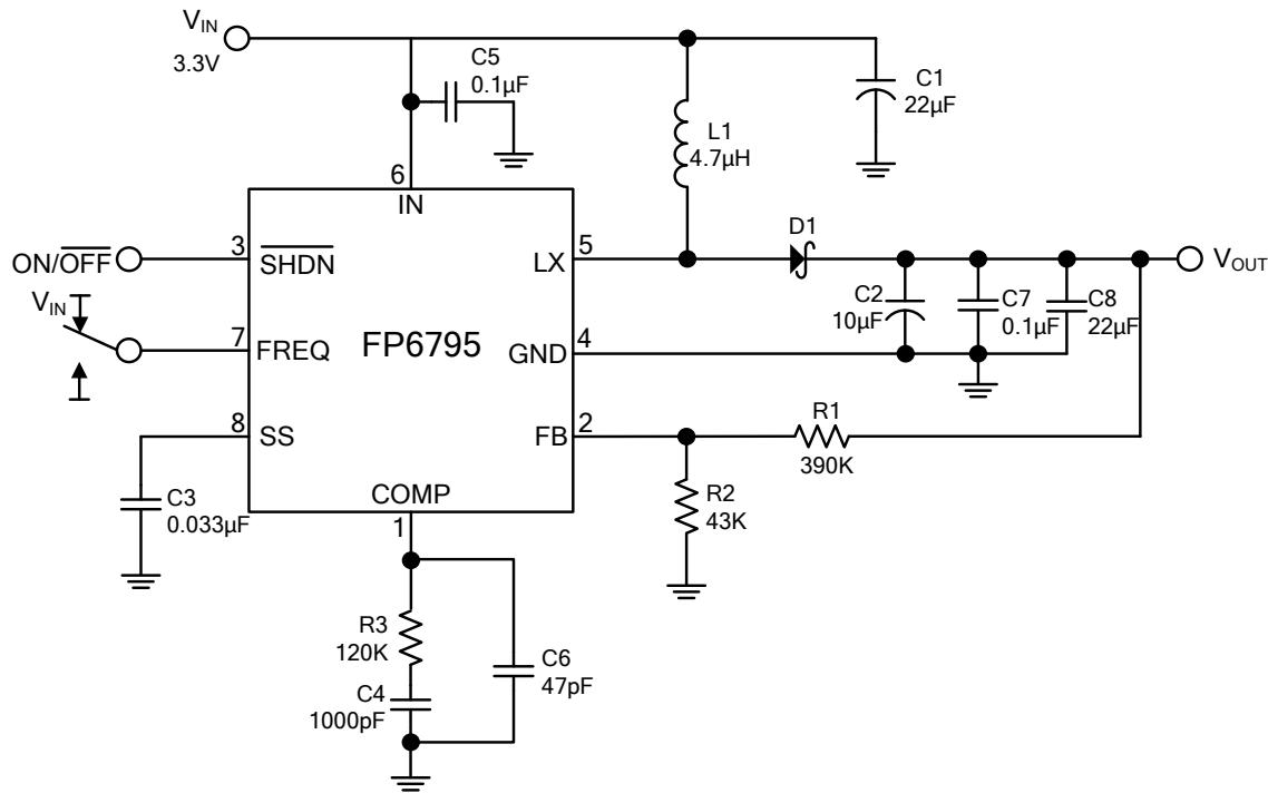
Figure 2. Typical Application Circuit of FP6795
