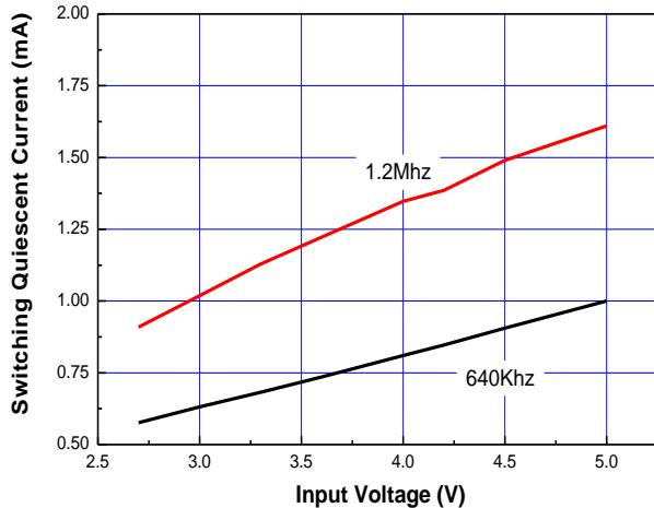
Figure 4. Switching Quiescent Current vs. Input Voltage
