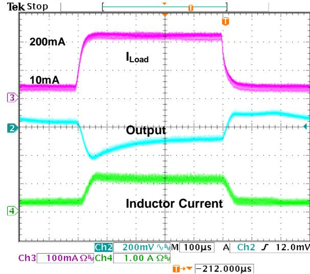
$V_{IN}=3.3V$ ,  $V_{OUT}=12.5V$ , FREQ=1.2MHz,  $C_{OUT}=33\mu F$
