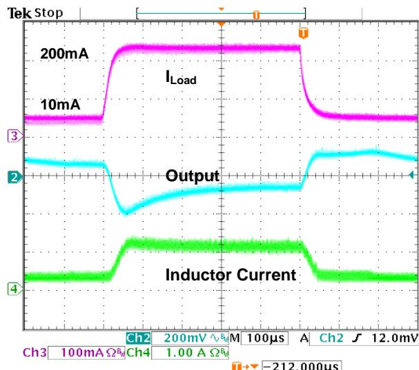
$V_{IN}=3.3V$ ,  $V_{OUT}=12.5V$ , FREQ=640kHz,  $C_{OUT}=33\mu F$
